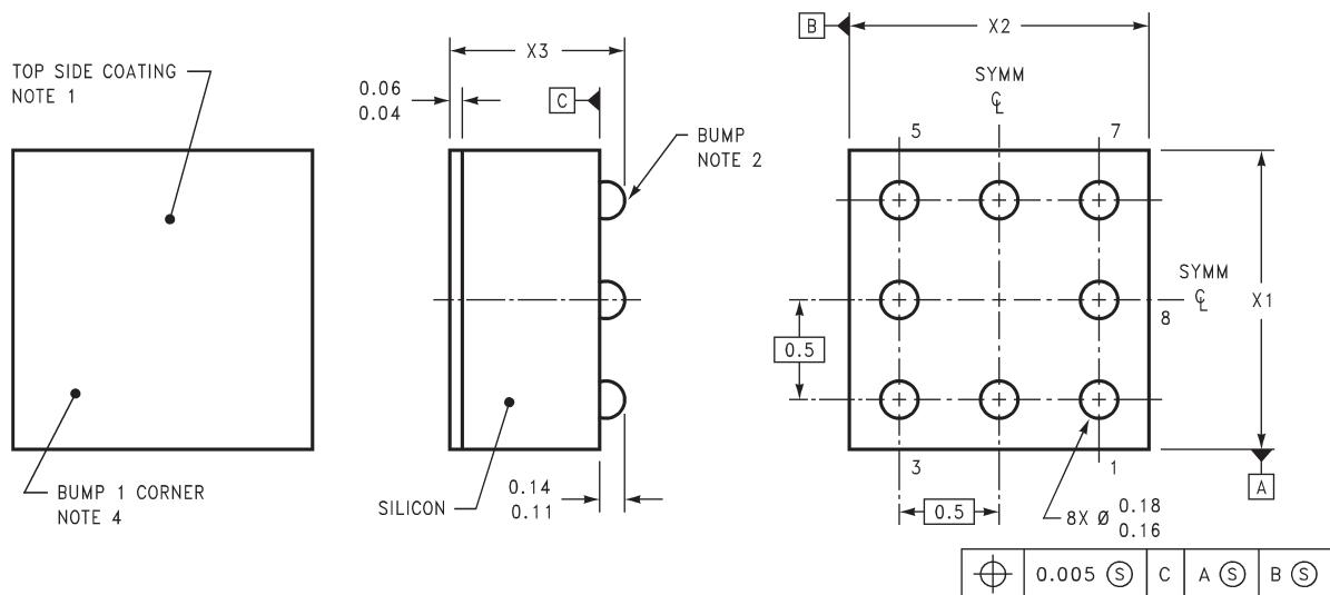
DIMENSIONS ARE IN MILLIMETERS
